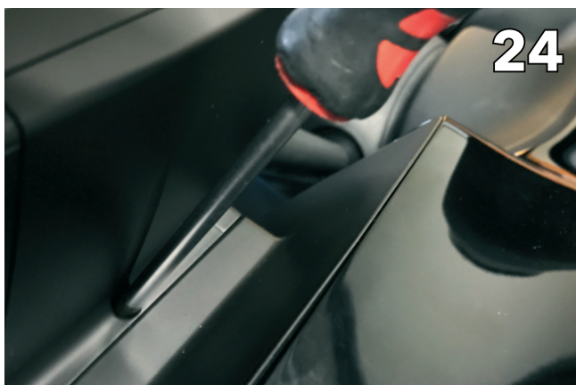
Slide the connector cover in the back of the screen and fix the screw (included with SPH-EVO93DAB-208)
