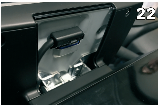
Insert the connector into the screen
