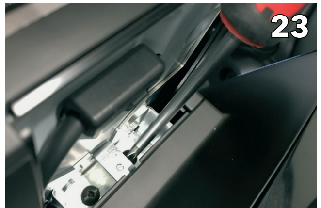
Slide the screen holder into the bracket and secure with two screws (included with SPH-EVO93DAB-208)
