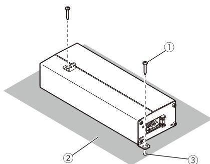
① Vis autotaraudeuses (4 mm × 18 mm )
