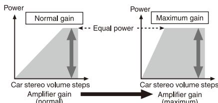
If amplifier gain is raised improperly, this will simply increase distortion, with little increase in power.
