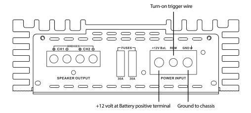
Note: The Z-Series AP amplifiers have terminals that do not require connectors. You simply insert a bare portion of wire and tighten the connection. As the wire conforms to the connector the connection can loosen. You should re-tighten the connection after about a week.
