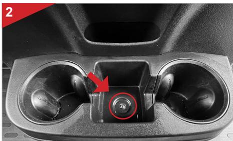
Remove the rubber insert in the center of the cup holder. Then loosen the screw (Torx T25) in the middle.
