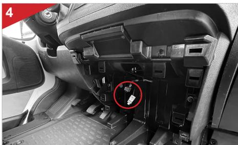
If present, pull out both connector plugs on the console and remove them completely.
