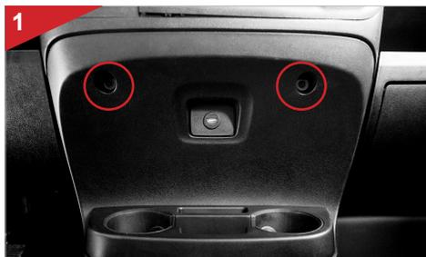
Loosen the two screws (Torx T25) above the cup holder.
