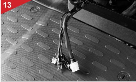
13 Connect the RCA connections and the turn-on wire to the radio/navigation system and route the cable including the bass level remote controller connection downwards.
