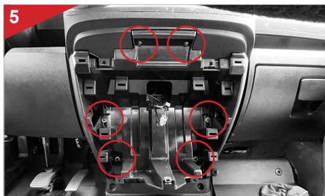
Remove the six screws (Torx T25) as marked above to be able to remove the console carrier.
