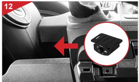
Now look for a suitable installation location for the included bass level remote controller, e.g. in the compartment to the right of the steering column.
