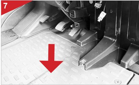
Now remove the cover in the footwell on the driver's side. The ten plastic screws can be loosened with a coin.
