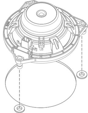
The OPTISOUNDMERC8WR/L-V2 subwoofer is a direct replacement for the factory fitted subwoofer. To Install, it will be necessary to remove the splashback cover in the front footwell. Once the factory subwoofer has been removed you can mount the OPTISOUNDMERC8WR/L-V2 subwoofer into the same location using the factory screw nuts.
