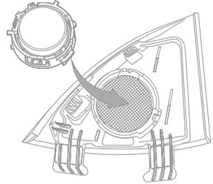
The OPTISOUNDMERC4C-V2 midrange is a direct replacement for the factory fitted midrange driver. To Install, locate into the three mounting sockets after removing the factory midrange.
