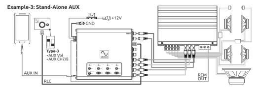
**Note:** For stand-alone systems where only the AUX input is used, select system Type-3 at the multi-function remote. This disables the remote's source select function and sets knob priority to master volume control for AUX input. Portable devices such as smartphones or MP3 players typically have an output voltage of 1Vrms or less, so it is recommended to maximize the device's unclipped output level and use the remote for the system's master volume.
