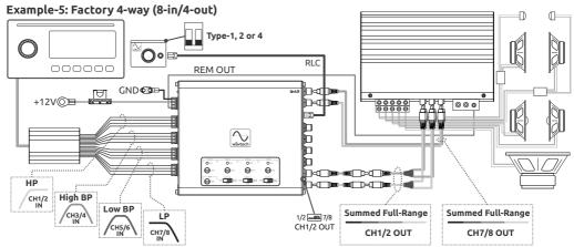
**Note:** The link8 can sum up to 4-way factory systems to full-range while also retaining independent remote level control over CH1/2 and CH7/8 outputs. If using the remote, choose the appropriate system type (see pg4) and set CH1/2's output select switch to 7/8 for a separate full-range output for main speakers and use CH7/8's output for subwoofer(s).
