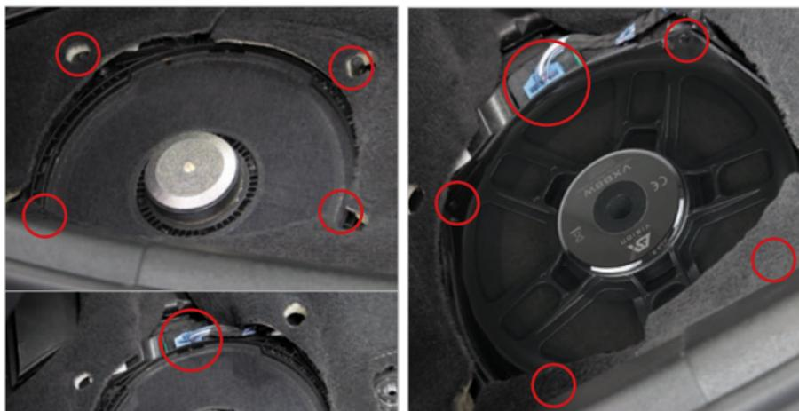
Now remove the original subwoofer, which is also attached with 4 screws, and disconnect the original cable plug. Then replace the original subwoofer with the ESX subwoofer, connect it with the original cable plug and screw it tight with the 4 original screws.
