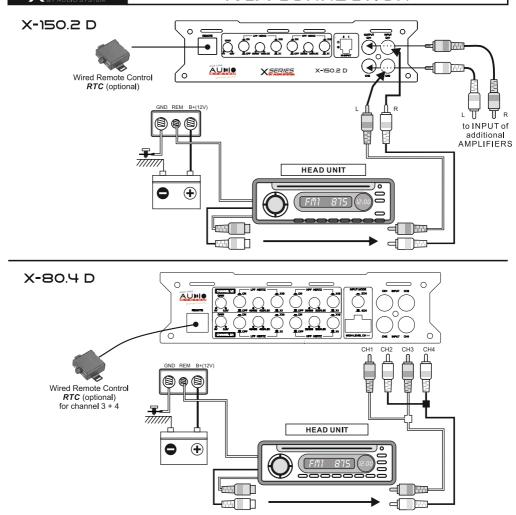
The X SERIES amplifier offers RCA-Inputs, which are connected through cinch cables with the preamplifier-outputs of the head unit. If the head unit (OEM-RADIO) has no RCA-Output, than it is possible to connect the speaker output direct to RCA/Cinch-Input. Important: the Gain-Controller has to be adjusted to minimum, then carfully turn up the volume. Input Mode has to be switched on "HI". If signal is presented, the amplifier automacally turns on.
