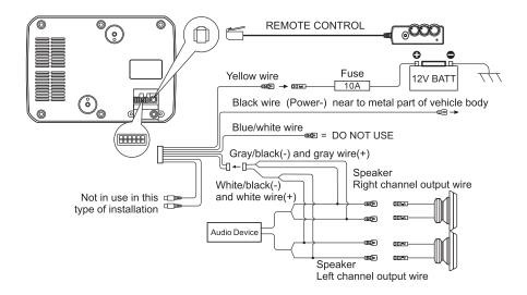
Wiring Diagram2 (Low level 'RCA' input)
