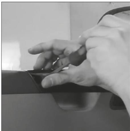
Remove the two screws from the door handle.
