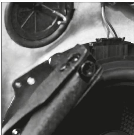
Attach the speaker using a hand riveter and six suitable rivets.
