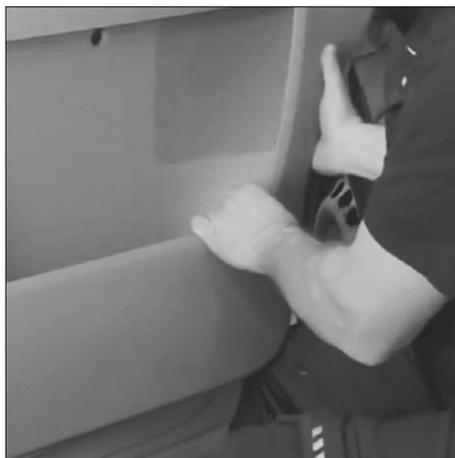
Unclip the door panel at the bottom and then carefully lift it out.
