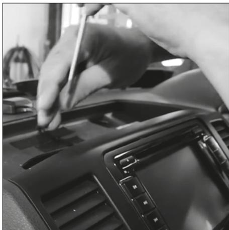
Then remove the car radio from the radio slot.
