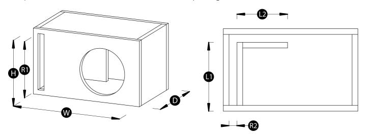
Note: Dimension are assume with 3/4" material (19mm). This is the suggested thickness. Less thickness may compromise box rigidity with leak bass response.
