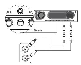
All RCA Inputs must be connected for the 2 channels work, including the Bridge Connection
