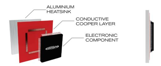
The **DTR**\* is a dynamic thermal recovery system which always maintains a high efficiency of the amplifier by accelerating the thermal exchange of electronic components with the heatsink
