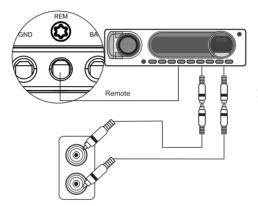
All RCA Inputs must be connected for the channel work.
