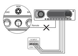
All High signal Inputs must be connected for the channel work.
