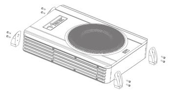
2. Screw the enclosure to the desired mounting location ensuring that there are no electrical cables, fuel lines or brake lines that may be damaged in the chosen location.
