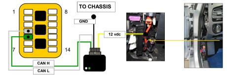
The second section of the harness is a kind of extension long 5 mt that must to lay down till the boot where is located the parking sensors device.
