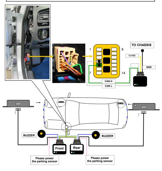
Attention: Use the PARKVIEW buzzer! Don't install the Park kit one The harness supplied with PARKVIEW is split in 2 sections; the first is composed by 4 wires to connect back plastic panel on DRIVER side of the vehicle.
