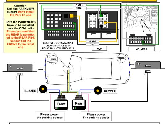
The harness supplied with PARKVIEW is split in 2 sections: the first is composed by 4 wires to connect back the OEM radio of the vehicle.
