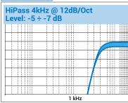
ATTENTION: Tweeter phase must be reversed by DSP setting for this set-up.
