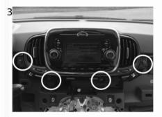
3 Unscrew, remove and save the dashboard air-vents as shown in the picture.
