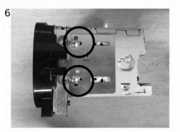
6 Take the new head-unit and fix the facia plate with the brackets as shown.
