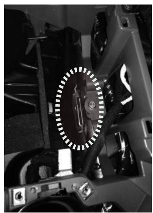
In order to place the aftermarket unit, cut the central metal bracket welded to the tube.
