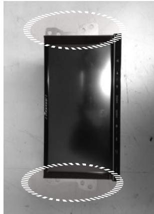
Place them as shown in the picture. Connect all cables, verify the proper functioning of the system and insert the unit into the housing. Fix it with screws saved before.
