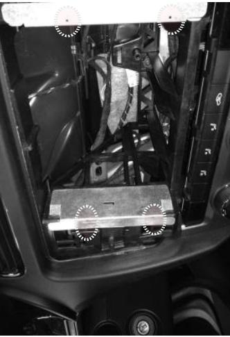
Connect all cables, insert the AFT unit into the housing and verify the proper functioning of the system. Finally fix all the brackets using the four small screws in the positions circled in the image.
