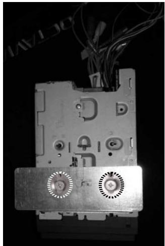
Take the remaining two brackets and mount them on the AFT unit using the screws supplied, slightly forcing them to indent the head of the screw.
