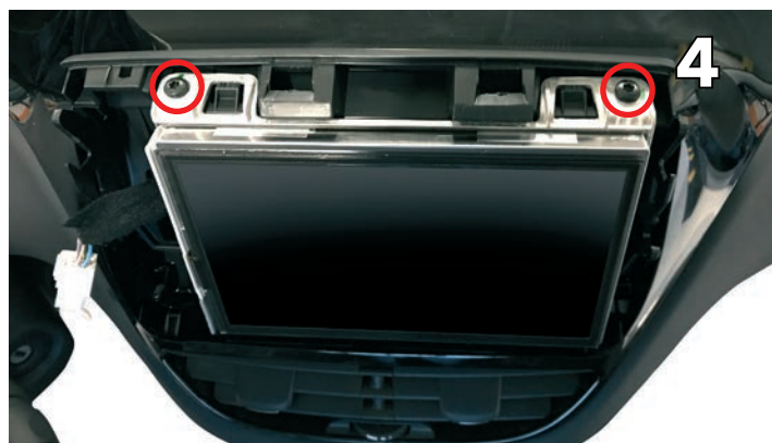
Remove two Torx screws on top
