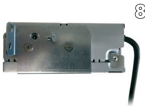
Mount the unit supports as shown by using the countersunk screws (supplied with the Pioneer product)
