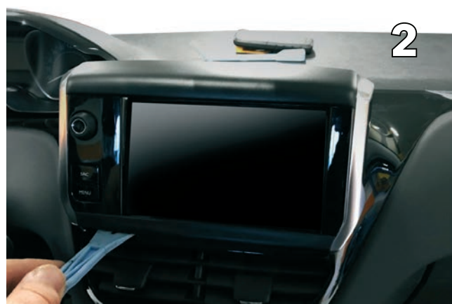
Remove front cover by lifting up as shown
