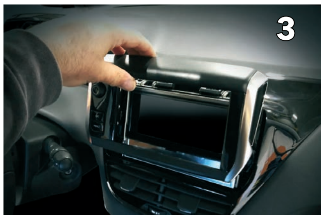
Pull upwards to remove and disconnect buttons
