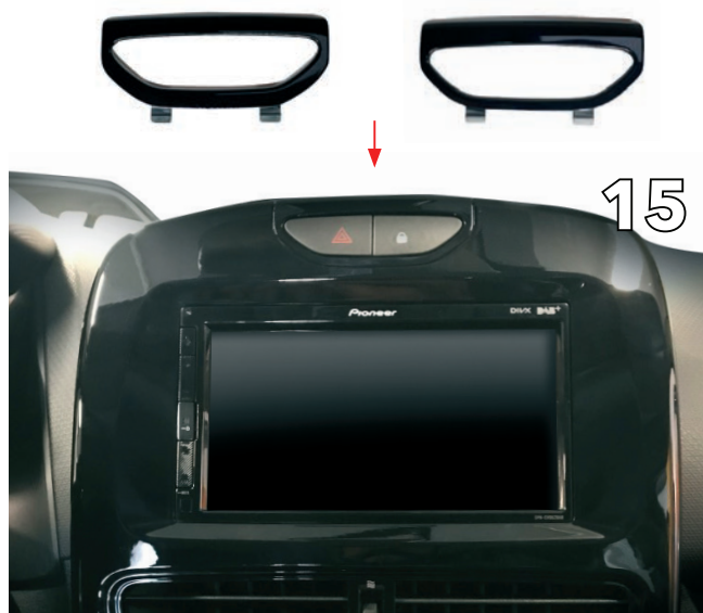
Put the fascia into the car and click the correct hazard switch cover in position
