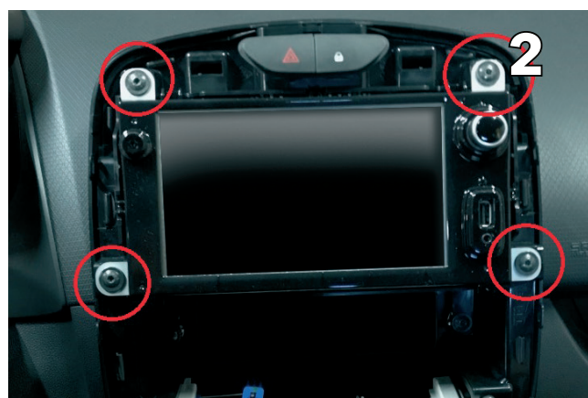
Remove the four indicated screws and take out the OEM receiver
