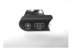
2) Remove the front plastic cover by pushing the lateral hooks and remove the original PCB.
