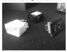
**Save** the white plastic after removing the PCB.
