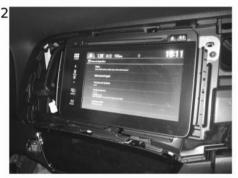
2 Remove the air vents and the dashboard. Unscrew and remove the head unit.
