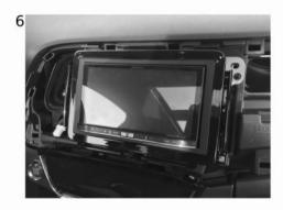
6 Connect all cables, verify the proper functioning of the system, put the new radio unit into the dashboard and fix it by screws.
