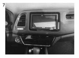
7 Put back in place the air vents, the dashboard and insert the facia plate. This is the final result.
