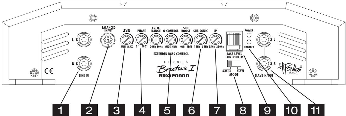
**1** The **LINE IN** RCA jacks must be connected with the RCA output jacks of the headunit.
