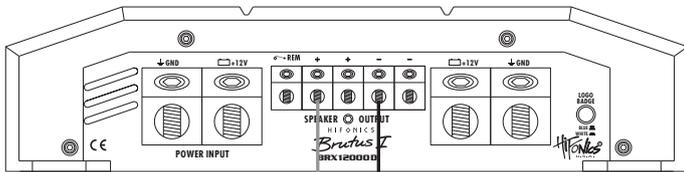
⚠ An additional subwoofer can be connected to the non-occupied speaker outputs. In this case ensure a impedance of 2 - 8 ohms per subwoofer.
