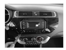
Remove the original panel, unmount the air vents; If the car is equipped with Start and Stop engine, unmount the button.
