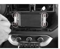
Before insert the radio pull down the internal bracket of the radio tunnel as shown in the picture.
