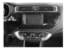
Place the clips saved before on the facia plate supplied, mount the air vents. If the car is equipped with Start and Stop engine, mount the button into the appropriate hole, otherwise install the cap with the two supplied screws. The image shows the final result.
