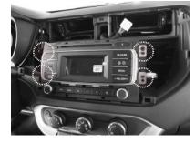
Unscrew and save the 4 screws of the original radio as shown in the picture.
