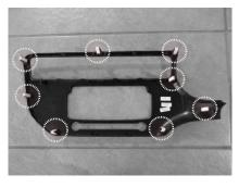
Remove and save the clips from the original panel as shown in the picture.
