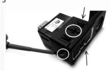
3 Take the original part and, in order to unhook the rear plastic, use a screw driver to carefully push the four holes indicated in the picture with circles and arrows.
