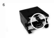
6 Disconnect the harness from the supplied PCB. Insert the PCB into the plastic part in the right position as shown. Plug back in the harness that you previously disconnected.
