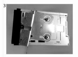
3 Put the mounting brackets on the head unit and fix them with screws. Pay attention to the letters on the brackets.with screws as shown in a photo.
