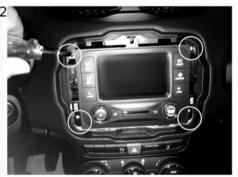
2 First: remove the original facia plate; Second: unscrew the screws from the dashboard and remove the original head unit.
