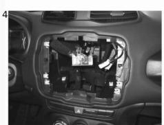
4 Connect all cables, verify the proper functioning of the system and insert the AFT head unit into the housing.
