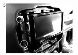
5 Adjust the AFT unit and fix it to the dashboard with screws.
