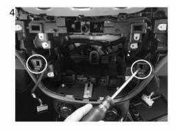
4 Remove the metal clips as shown in the picture.
