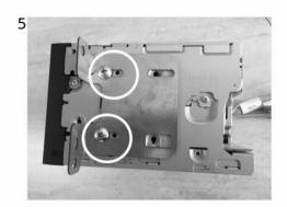
5 Take the supplied brackets and fix them to the head unit as shown in a picture.
