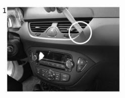
1 This is how the original dashboard looks like. Remove the cover as shown in the picture.
