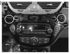
2 Remove the facia plate by unscrewing the circled screws as shown and save the buttons.
