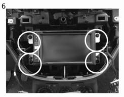
6 Connect all cables, verify the proper functioning of the system, put the new radio unit into the dashboard and fix it by screws.
