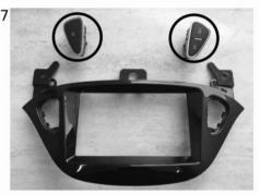
7 Insert the buttons previously saved in the supplied facia plate.
