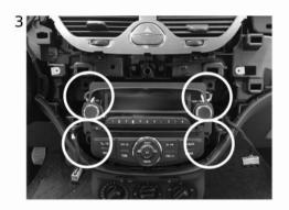
3 Remove the head unit by unscrewing the circled screws as shown and save them.
