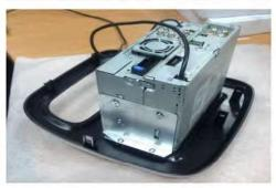
6. Once all the connections are in place, insert the new Radio carefully in the dash to avoid damage to the leads. We recommend to try the Radio is working before the screws and fascia are fitted
