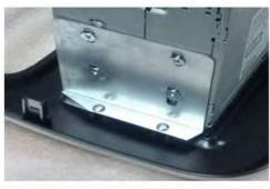
5. Attach the brackets to the Radio and Fascia
