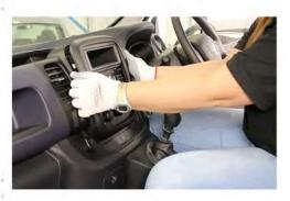
7. Attach the metal clips to the fascia. Align the fascia to the holes in the dash and press in firmly.
