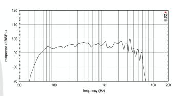
FREQUENCY RESPONSE MADE IN 60 LT. ENCLOSURE TUNED AT 50 Hz IN FREE FIELD (4pi) ENVIRONMENT.
