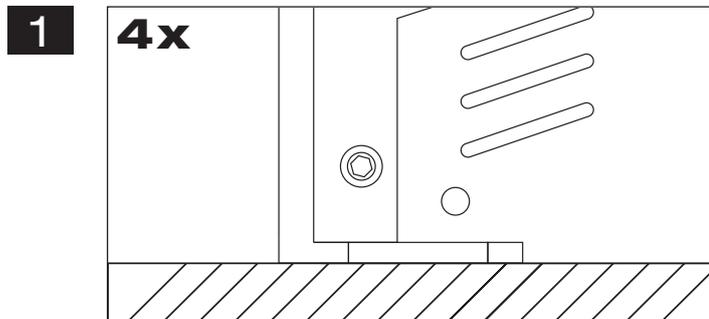
**1** At first you need to find a suitable installation location for the amplifier. Ensure that enough space for the installation of the cables remains and that they will not be bended and have sufficient pull relief.
