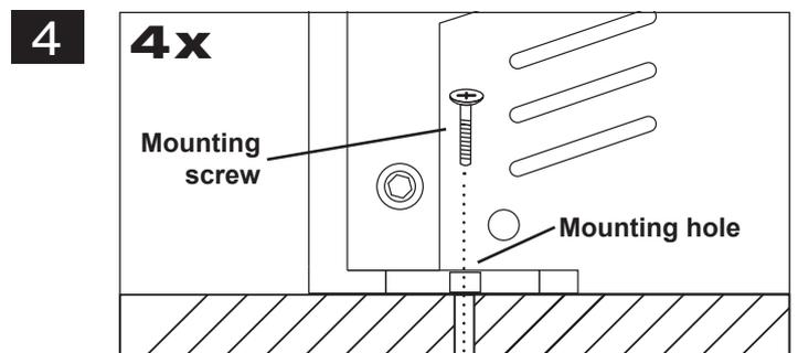
**4** Then uphold the amplifier to the chosen position and fix the screws through the mounting holes into the drilled screwholes.
