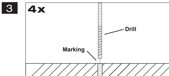
**3** Lay the amplifier aside and then drill the holes for the mounting screws at the marked locations.
