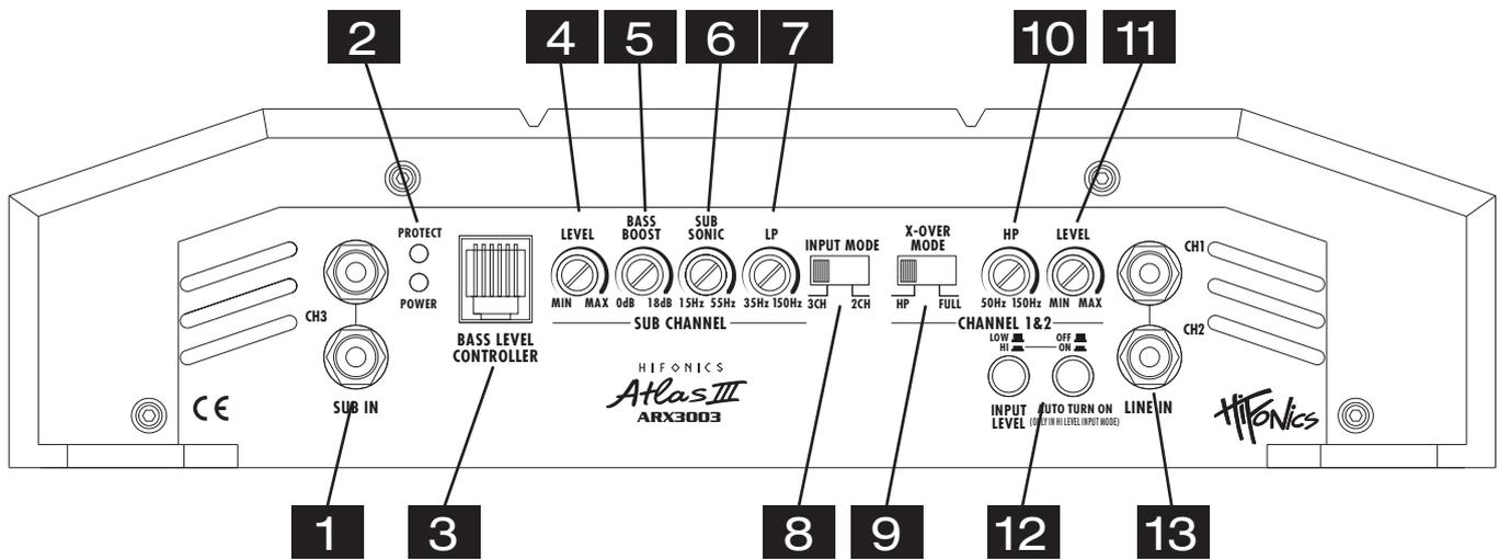
**1** The **SUB IN** RCA jacks must be connected with the RCA output jacks of the headunit. Please check also the notes in section #8 below.
