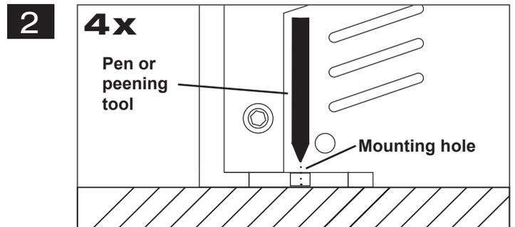
**2** Keep the amplifier at the chosen mounting location in the vehicle. Then mark the four drill holes with an appropriate pen or peening tool through the designated mounting holes at the amplifier.
