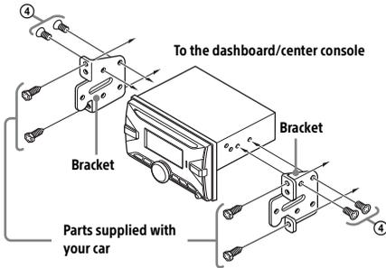
When mounting this unit to the preinstalled brackets of your car, use the supplied screws ④ in the appropriate screw holes based on your car: T for TOYOTA and N for NISSAN.
