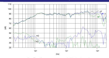
Note: Filtered frequency response measured with loudspeaker standing on infinite baffle in anechoic chamber, 1W @ 1m with FD-2CX/Fe
