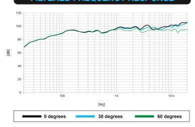
Note: Filtered frequency response measured with loudspeaker standing on infinite baffle in anechoic chamber, 1W @ 1m using filter FD-2XA
