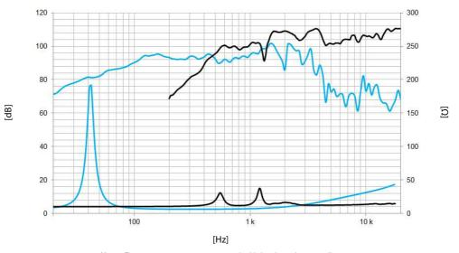
Note: Frequency response measured with loudspeaker standing on infinite baffle in anechoic chamber,  $1\dot{W}$  @ 1m
