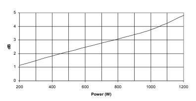
Note: Power Compression Losses were calculated after 5 minutes period applying a pink noise signal filtered between 40 and 200 Hz.
