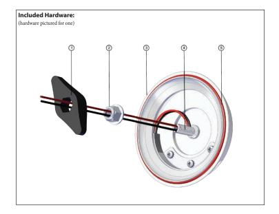
NOTE: The M-LCA-C-W Light Cap and M880-ETXv3-SG-WH Enclosed Speaker System are used in this manual for illustrative purposes only. The installation steps are the same for all ETXv3 and VeX<sup>™</sup> Enclosed Speaker Systems and all LED Light Caps.
