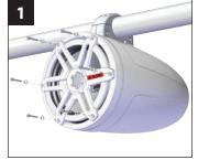
Remove the six #8 x 1-1/4" Pan Head Screws and six #8 Flat Washers that secure the speaker to the enclosure.
