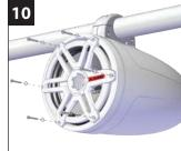
Reconnect the speaker wiring, and reinstall the speaker using the six #8 x 1-1/4" Pan Head Screws and six #8 Flat Washers.
