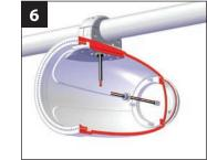
Slide an M10 x 1.5 Nylon Insert Flange Locknut over the LED wiring, and hand-tighten onto the Threaded Stud.
