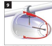
Connect the LED wires from the LED Light Cap to the LED wires entering the enclosure. Refer to the wiring charts on the opposite page for details. DO NOT install the fuse holders inside the enclosure.
