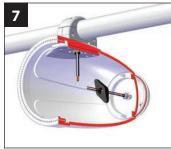
Slide the M10 Locknut Tool over the LED wires and onto the M10 x 1.5 Nylon Insert Flange Locknut.
