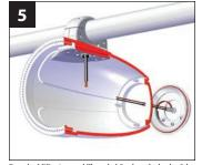
Pass the LED wires and Threaded Stud on the back of the LED Light Cap through the drilled hole, and position the cap flush against the back of the enclosure.
