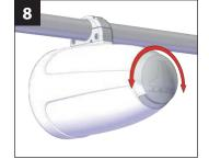
Rotate the LED Light Cap to the desired angle. Using the M10 Locknut Tool, fully tighten the M10 x 1.5 Nylon Insert Flange Locknut until the O-ring is fully compressed and not visible to ensure the unit is properly sealed. Remove the M10 Locknut Tool from the enclosure.
