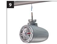
Have a helper support the enclosure during this step. Use the supplied butt connectors to connect the red (+) and black (-) speaker cable exiting the ETXv3 enclosure to the speaker cable exiting the pipe. The green and white wires will not be used in this application.
