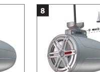
Apply Loctite® red thread-locking compound (included) to two 5/16" - 18 x 1-1/4" machine screws (included), thread them into the base of the fixture, and push down on the fixture to ensure no gap while fully
