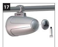
For best adhesion, it is recommended to clean the inside of the aluminum cap with acetone (not included), prior to attaching it to the speaker enclosure. Apply a circular bead of silicone adhesive (included) to the inside of the aluminum logo cap, about 1/2-inch (13 mm) from the outer edge.
