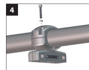
Determine the speaker mounting location, and temporarily secure the fixture around the pipe by hand tightening the four 1/4 - 20 x 1-1/4" machine screws and
