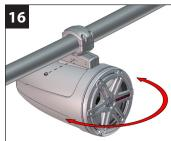
Rotate the enclosure to the desired angle, install the 5/16 - 18 x 1/2" set screw into the base of the fixture, and
