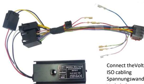
Connect the Voltage converter between the ISO cabling
