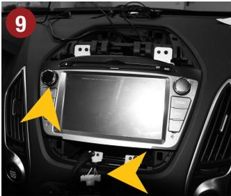
9.) Before you complete the installation, make a function check. Please note that it may take up to 15 minutes, until a GPS signal can be received outside.
