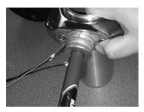
3 Drill a <sup>5</sup>/<sub>4</sub>" hole where the mark was made. The speaker wire/dome light and LED logo power wire will be passed through this hole. Place a grommet in the drilled hole so the wire will not be damaged by the sharp edge of the pipe.
