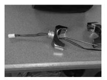
5. Attach the power and signal wires from the vehicle to the included wire harness that was pulled through the bottom bracket. Pull back the wires so only 2" of slack protrude from the bottom bracket. If too much wire is hanging out it won't fit well in the internal enclosure recess (the wire may bind and cause a short, take care to not get any wire caught in the locking mechanism).
