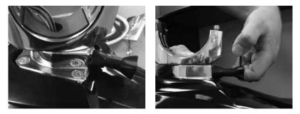
10. Tighten the locking knob by hand. Next use an 18mm open end wrench to tighten down the lock knob so it wont move. Using the 18mm wrench will ensure enough torque is applied to keep the unit from loosening.
