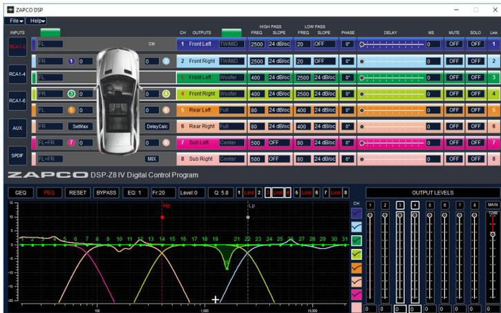
The user has found that the frequency cut at 1,600Hz is not quite right but it is close. Using the PEQ you can click on the filter number to activate it and then click into the Q box above and change using the up/down arrows in steps of 0.1. You can click into the Level box and use the arrows to change the boost/cut in steps of 0.5dB.
