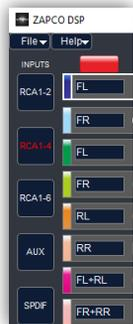
In 4-channel mode as on the left the front 4 channels are defaulted to 2 left and 2 right input channels to give highs and lows at the front and channels 5 and 6 are set to receive left and right rear channel inputs. Channels 7 and 8 will receive the sum of both front and rear inputs to give a summed bass or center channel as desired. In 6-channel mode channels 7 and 8 will be set to receive the last channels of input.
