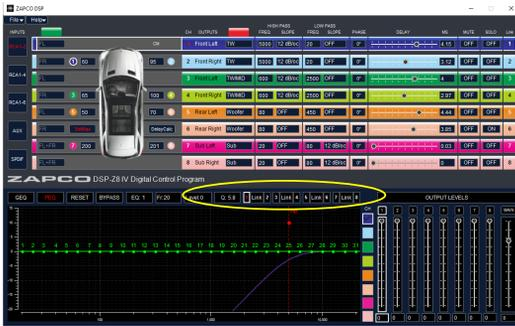
You click the Link between Ch1 and Ch2. It will ask you to confirm, then the link will turn red and the 2 channels will adjust together. In this case we will link all 4 channel pairs.
