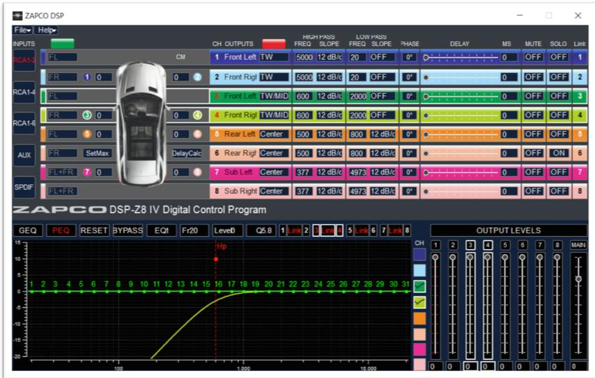
The top front section is where you make the basic set-up and you can see the entire system at-a-glance whenever needed.
