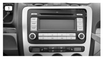
Gently lift the trim frame starting on the right side of OE device. For successful completion of this step, using a release tool made of plastic tool is mandatory.
