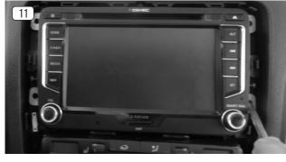
Neatly arrange the wires to the side, making room for the ZENEC system. Carefully slide it into the radio slot and fix it in place, using the four original Torx screws.
