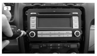
3. Unscrew and remove the four Torx Screws (T25) of the original device.
