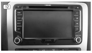
12. Press the trim frame back on to make the installation complete.
