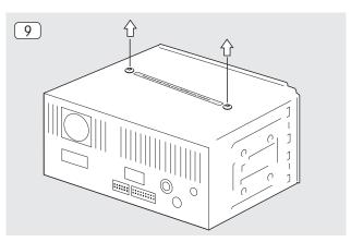
9. Before installing the ZENEC system (No. 1) remove the two transport securing screws.
