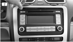
Run the prying tool anticlockwise around the trim frame, to release it from the console. The trim frame should come off of the console completely.
