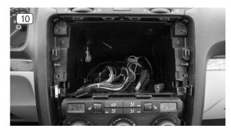
10. Connect all the cables to the ZENEC system (No. 1): those previously run in the radio slot, and the original antenna cables.
