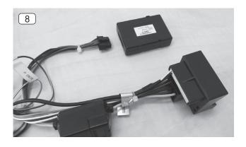
8. Connect one of the main connection cables (No. 5 or No. 6) of the ZENEC system (No. 1) to the Quadlock connector of the car and close its locking mechanism. Please pay attention to the compatibility list in this document to choose the suitable main connection cable, including in the delivery, for your vehicle. Following this, connect the CAN bus interface (No. 7) to the main connection cable.
