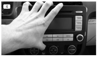
4. Remove the original device by pulling it out of the radio slot. Detach all the cables from its backside.
