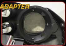
Align adapter with factory screw holes and attach with supplied screws. Be sure gasket is properly seated between grille and adapter.
