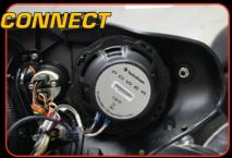
Install speaker using screws supplied with speaker and reattach speaker wires. Be sure to use proper polarity when connecting speaker. Test and reassemble fairing.
