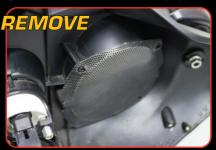
Remove fairing to gain access to speakers. Once removed, unplug and remove speakers and mounting ring. Retain factory woven speaker grille.
