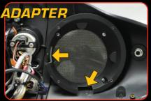
Align adapter with factory screw holes and attach with supplied screws. Be sure gasket is properly seated between grille and adapter. Example shown above is for speakers with bridge mounted tweeters. Use wire cutters and pliers to remove tabs. Apply gaskets to notches prior to speaker placement.
