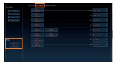
Several new features are visible in the DSP PC-Tool after installing a MEC module.
