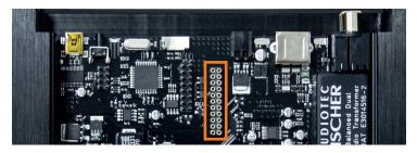
Make sure that the MEC module is installed properly and all pins are fully inserted into the socket:
