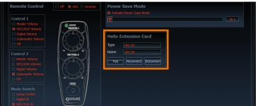
After the pairing mode is activated the Bluetooth® network can be found under the name "HEC BT". There is also the possibility to change the name by clicking on the name field of the HELIX EXTENSION CARD section of the DCM menu.
