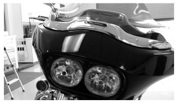
Leaving the windshield in place, remove the six inner fairing screws.
