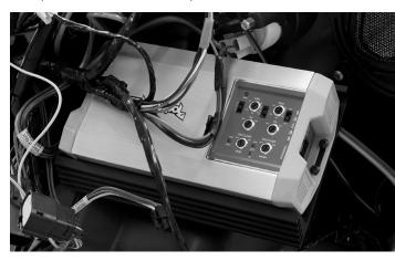
Once the amplifier is mounted, you can now begin plugging in the wiring harness in their appropriate sockets.
