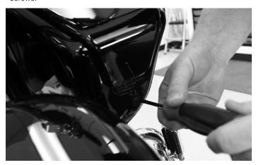
After the screws are removed, use your socket or ratcheting wrench to unbolt the turn signal brackets.
