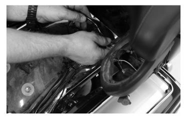
Unplug the factory speaker wires from the speaker and plug them directly in to the Rear Speaker Input / Output Harness. These are labeled clutch and brake side.
