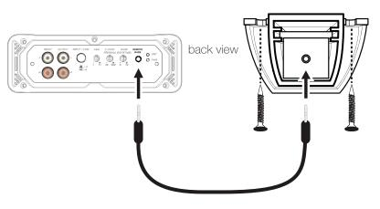
Connect the supplied 1/8th inch [3.5mm] patch cable to the CXARC remote and the Remote Bass jack on the amplifier
