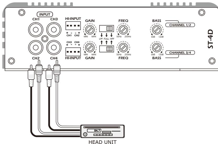
Connect your source unit to the amplifier using the "INPUT" RCA connectors. The "OUTPUT" connector can be used to pass the input signal to another amplifier. For Initial Setup: Always set bass boost to 0dB, and set the amplifier gain to minimum (8V sensitivity). Remember: amp gain is not a volume control. It is used only to match your amplifier input sensitivity to your source unit output.
