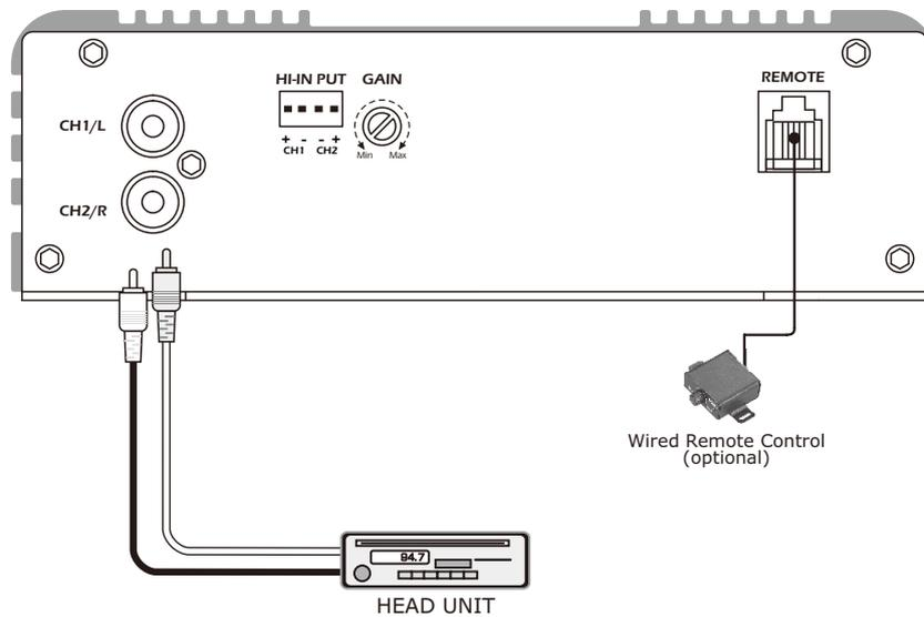
Connect your source unit to the amplifier using the "INPUT" RCA connectors.
