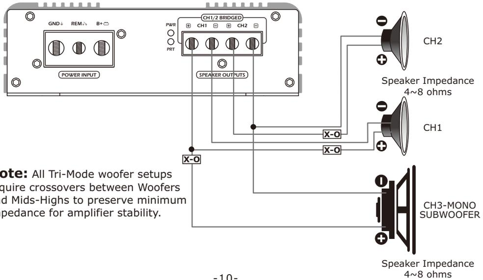
**Note:** All Tri-Mode woofer setups require crossovers between Woofers and Mids-Highs to preserve minimum impedance for amplifier stability.
