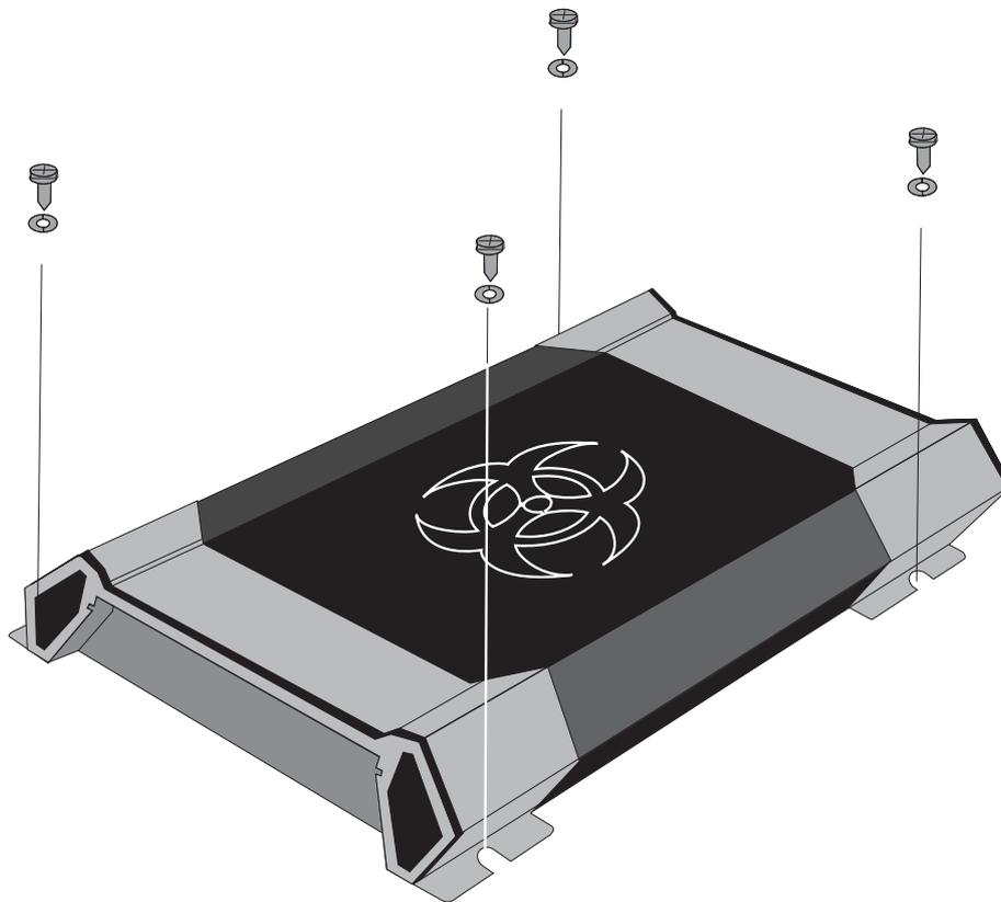
**1** At first you need to find a suitable installation location for the amplifier. Ensure that enough space for the installation of the cables remains and that they will not be bended and have sufficient pull relief.
