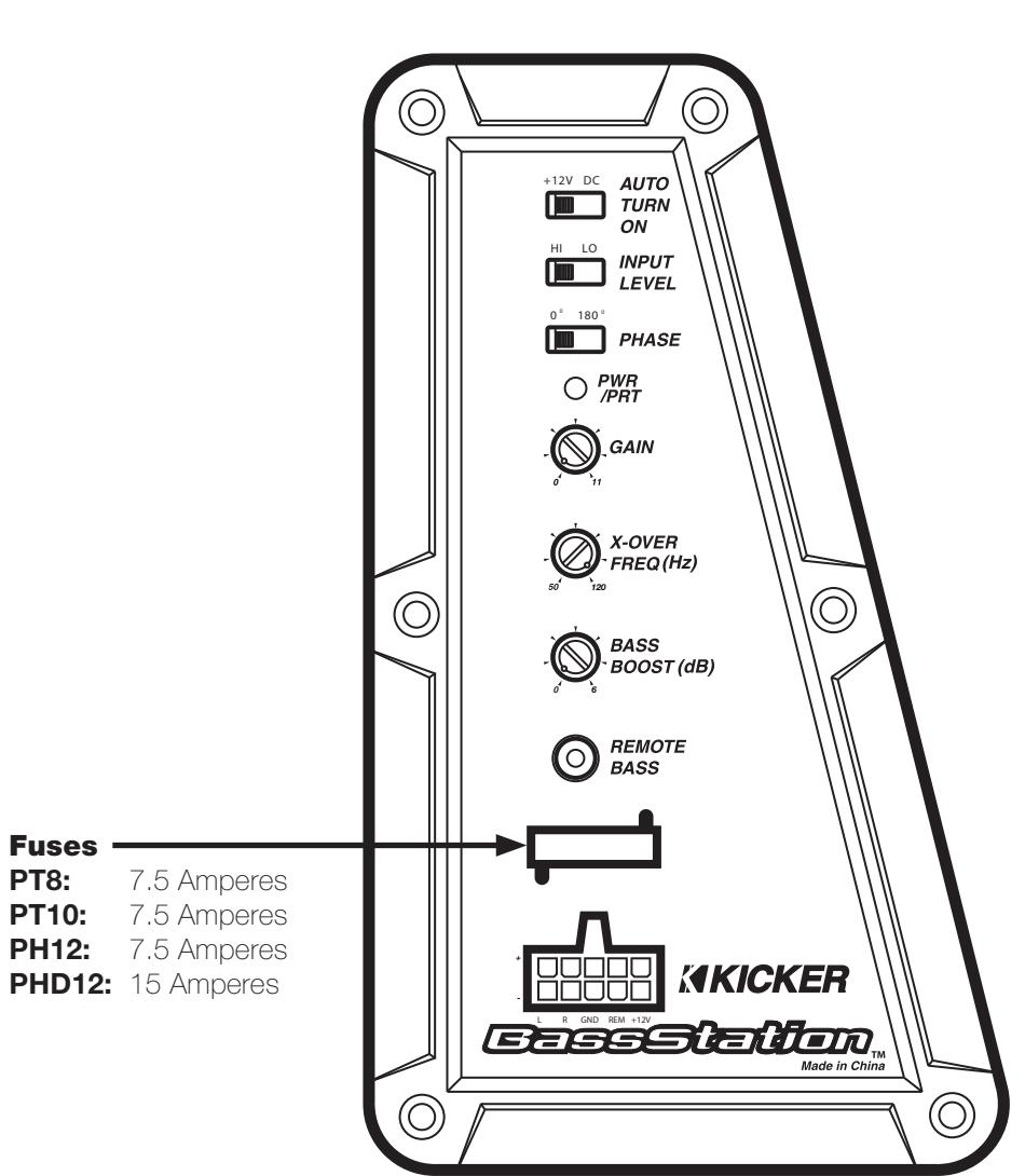
**Automatic Turn-On Selection:** KICKER powered enclosures offer two different automatic turn-on modes that can be selected on the side panel; +12V and DC Offset. Using the DC Offset mode causes the REM terminal to have +12V out for turning on additional amplifiers.
