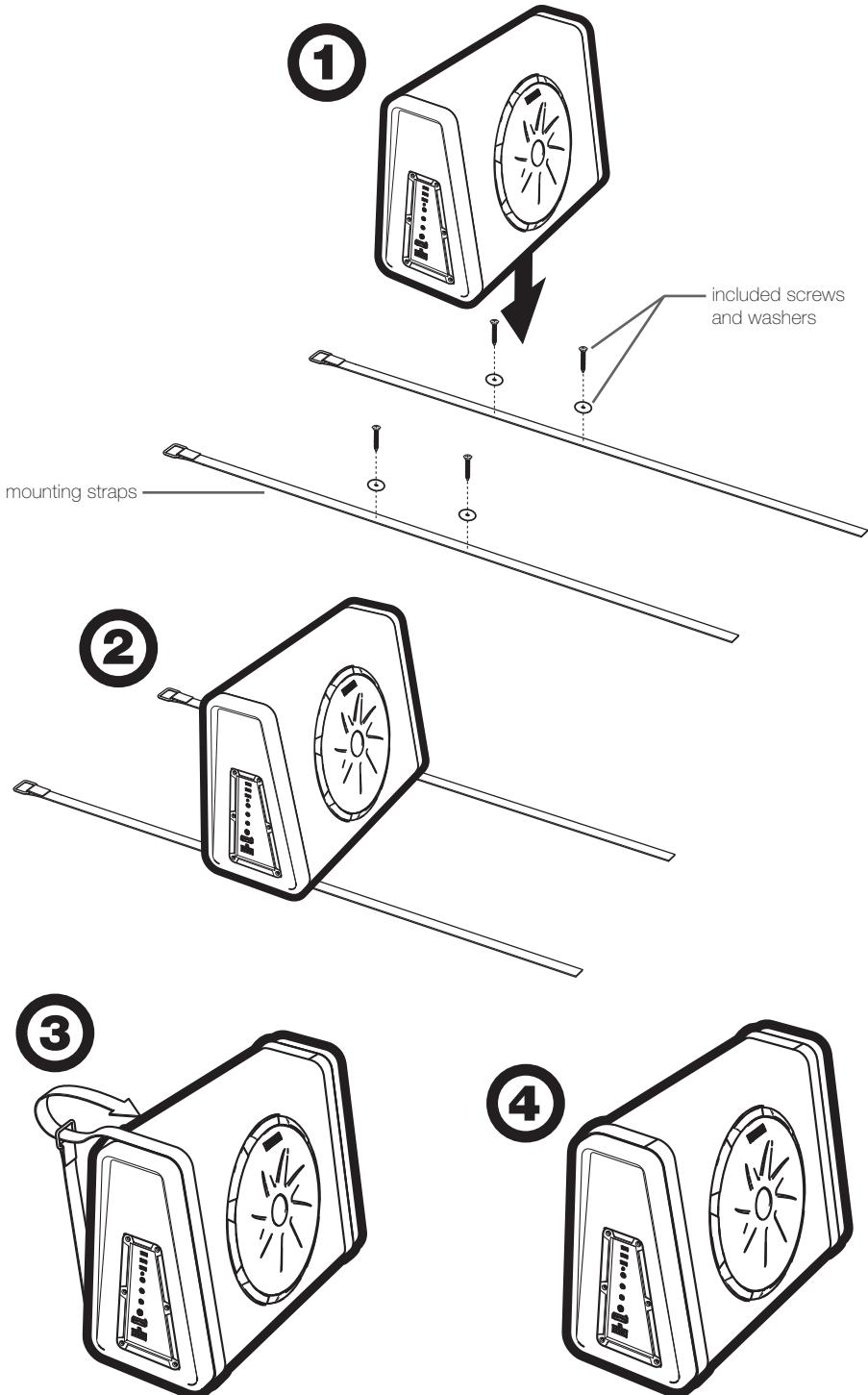
If the supplied mounting hardware is not applicable to your installation, some other means of securely attaching the enclosure to the vehicle must be used.
