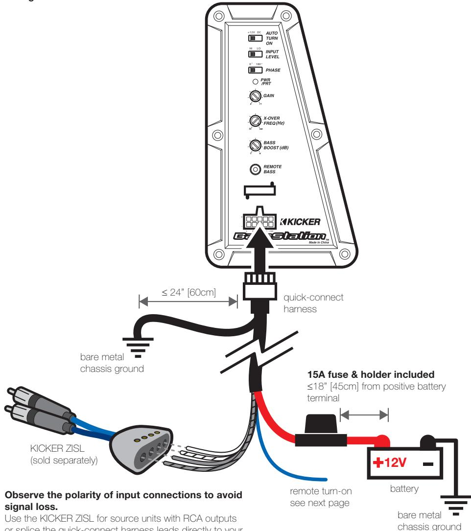
**Observe the polarity of input connections to avoid signal loss.**
